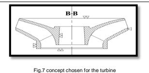
The liquid turbine communicates a part of the kinetic energy transmitted by the shaft through its blades (fins). It is mounted on the shaft of the pump by means of a cone and a nut (the method of fixing by adherence).
