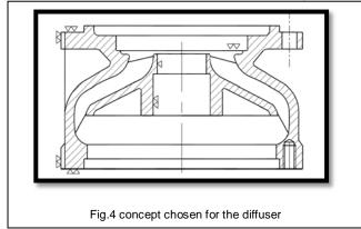
The diffuser is designed to collect the liquid coming out of the wheel, and the direct or to the discharge port, either to the input of the next wheel, depending on whether the pump is single or multistage.
