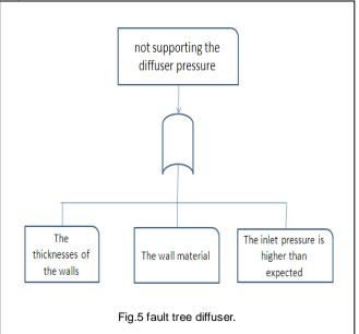
From Figure 5 and to eliminate the causes of the failures we have adopted the following solutions
